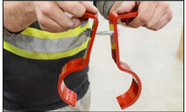
Fig 45 - 2 inch bolt joining the brackets
