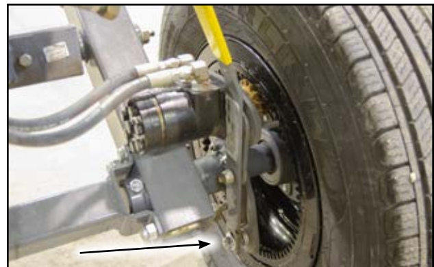
Fig 38 - Flange nut at bottom of assembly
