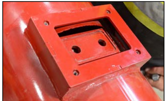
Fig 46 - Hanger bearing with Spacer Cover Plate
