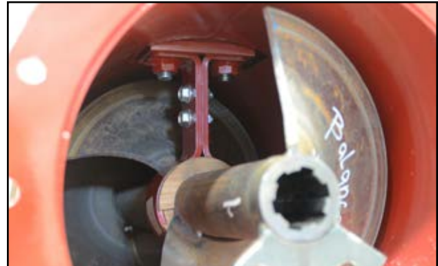
Fig 28 - Hanger bearing from end of tube
