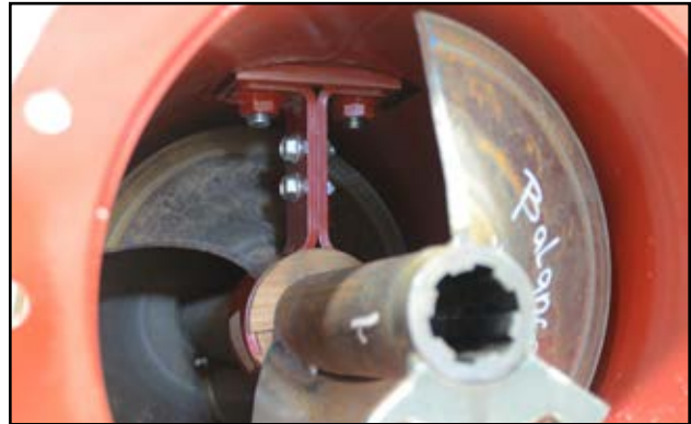
Fig 42 - Hanger bearing installed inside tube
