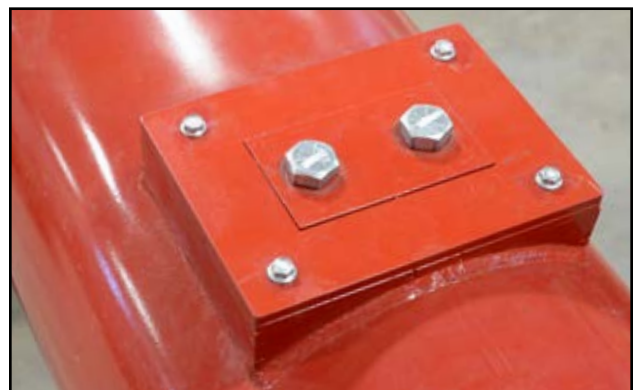
Fig 47 - Cover Plate covering Hanger Bearing
