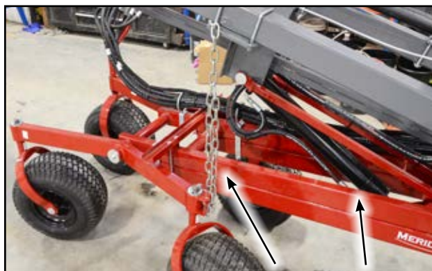
Fig 17 - Walking Beam transport chain and lift cylinder
